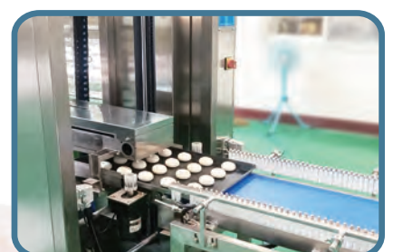
烤盤進入盤台車系統 Tray is sent to the Auto. Tray-Input Trolley System
