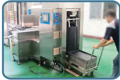
手台車送入補盤機 Hand-Trolley is fed to the Tray Supplying Machine
