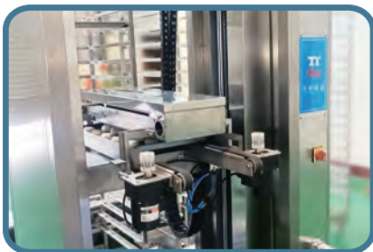
烤盤預備插入台車 Tray is ready to insert to the trolley
